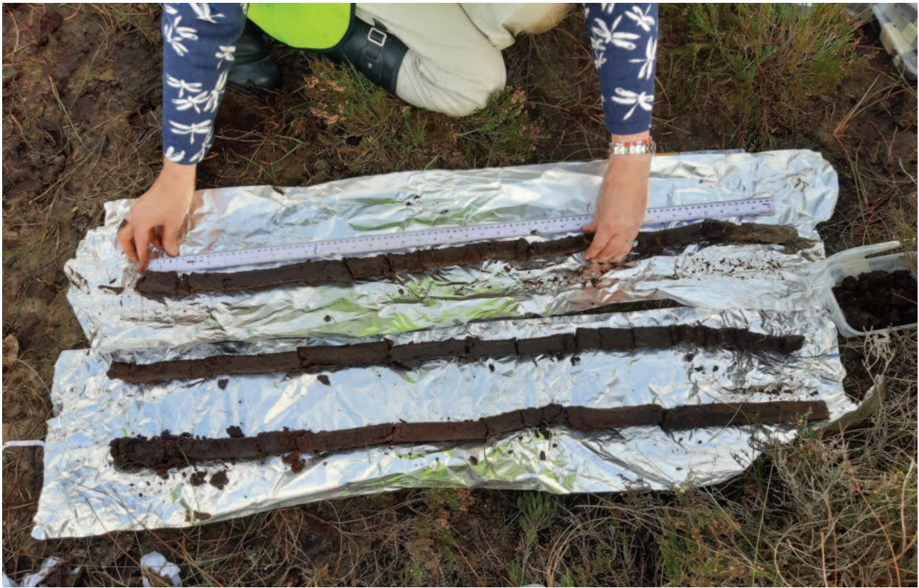
Figure 7: Peat core measuring 3m removed from Girley Bog, Co. Meath for stratigraphy and bulk density determination in 2020. The changing colours and textures of the peat within the core represent different types of peat laid down in the history of the development of this site. Photo: © N. Madigan
