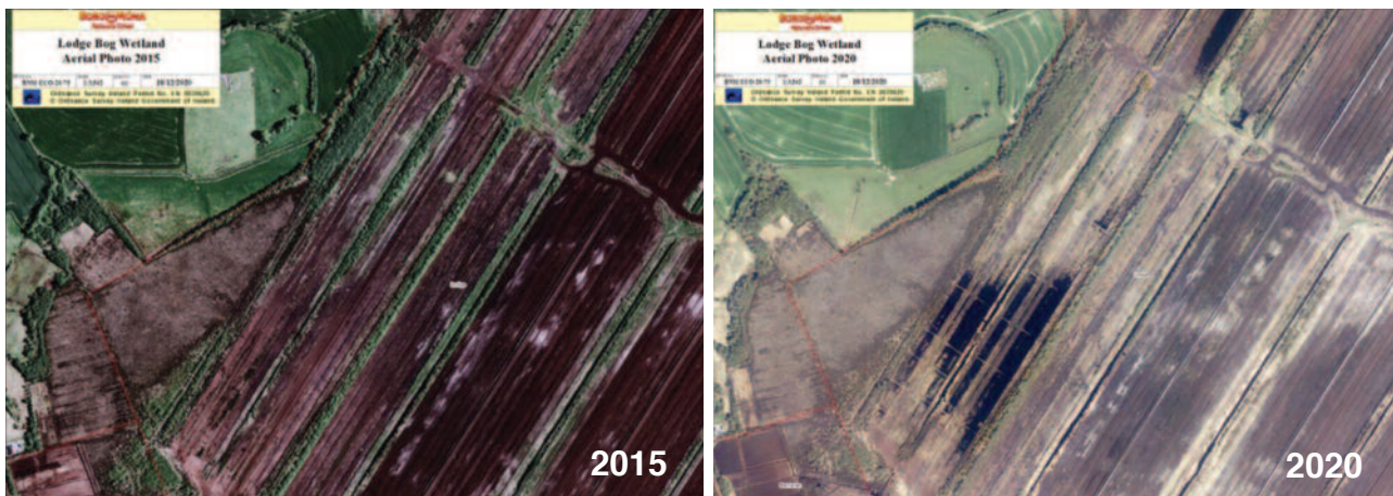
Figure 20: Hydrological images for Lodge Wetlands South, Co. Kildare from 2015 (left) before rehabilitation began and in 2020 (right) showing rewetting of the residual peat through the creation of berms and blocking the outflow from the site. In managing for climate change it is necessary to rewet a greater proportion of such sites through reprofiling of the peat surface remaining in the post-industrial site. Photos: © Bord na Móna
