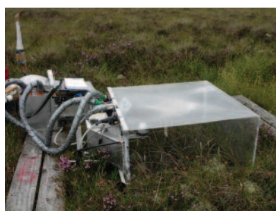
Figure 15: "Clear" chamber on Clara Bog, Co. Offaly used to measure net exchange of CO 2 between an ecosystem and the atmosphere (NEE). Photo: © D. Wilson
