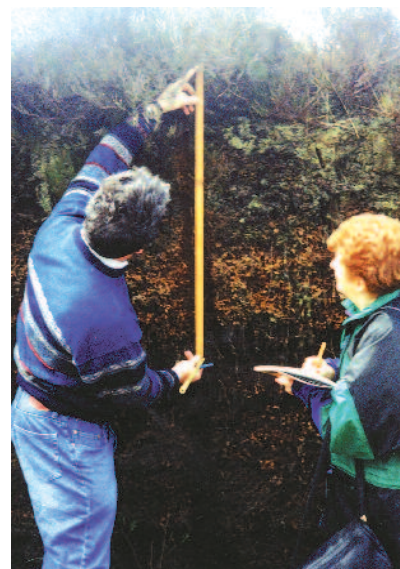
Figure 2: Measuring the extent of the younger and older Sphagnum layers visible in a peat bank left behind by turf cutters on a raised bog at Croghan, Co. Roscommon. The peat accumulates at a rate of 1mm per year and may store 2 up to 1314 t C ha -1 . Photo: © C. O'Connell
